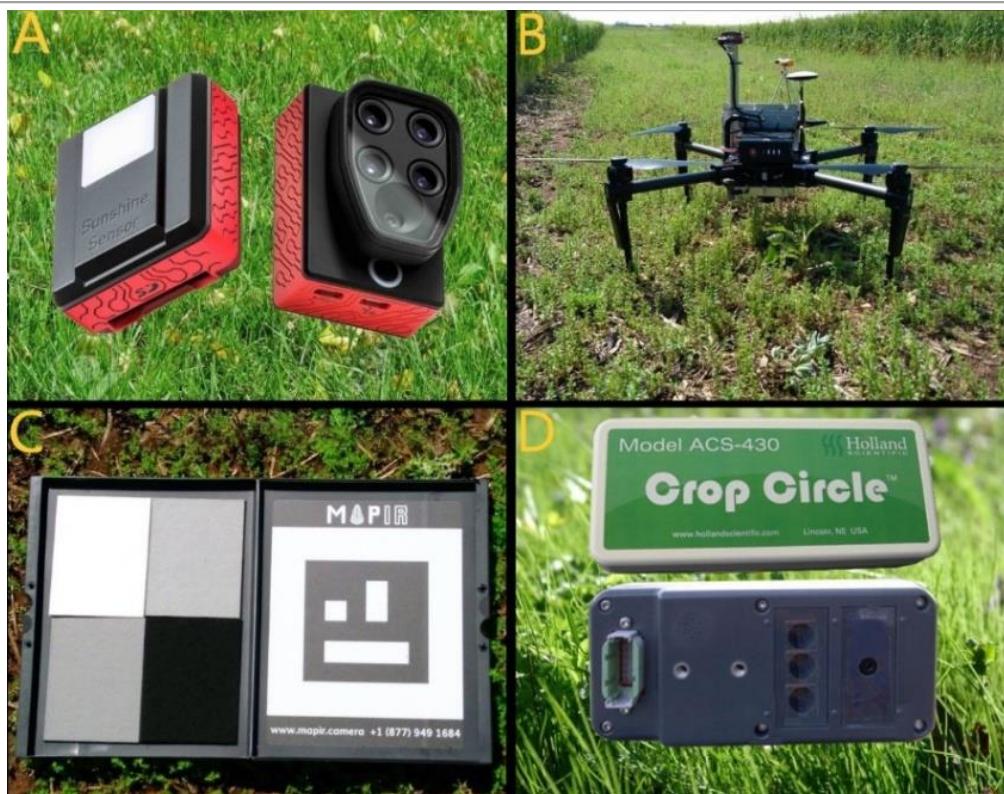
FIGURE 1. Equipment used in this experiment: (A) Sequoia camera; (B) DJI Matrice 100 UAV; (C) MAPIR V2 reflectance calibration ground target; (D) Crop Circle ACS-430 ® sensor.
