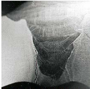
Figure A10.1 IGSCC of piping welded joints heat affected zones (HAZ)
