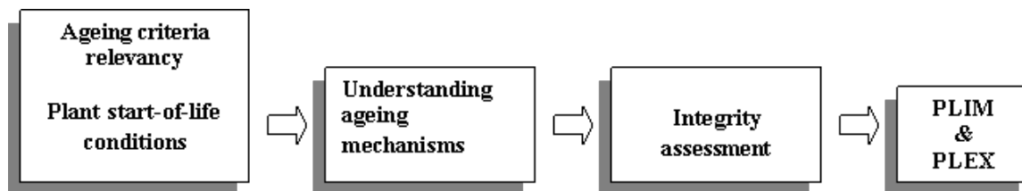
Figure A17.2 Typical goals of the material ageing management of carbon and austenitic steel pipes in PLIM/PLEX programs.
