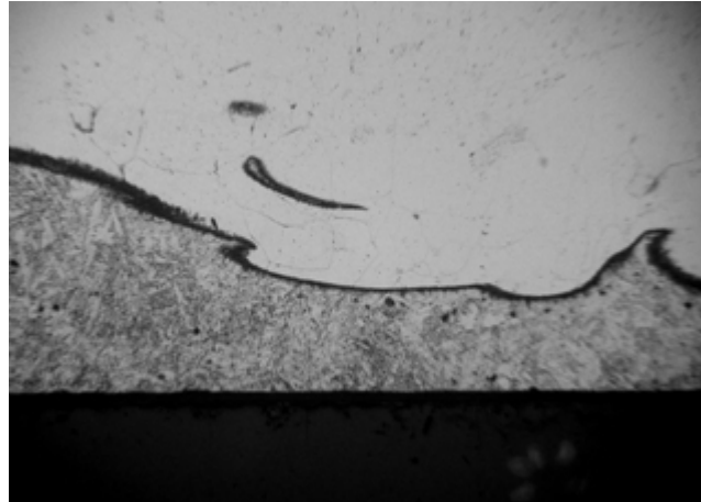
Figure AN.1.6 Small slag inclusion in the first layer of the cladding (N=100x) [AN1.1]
