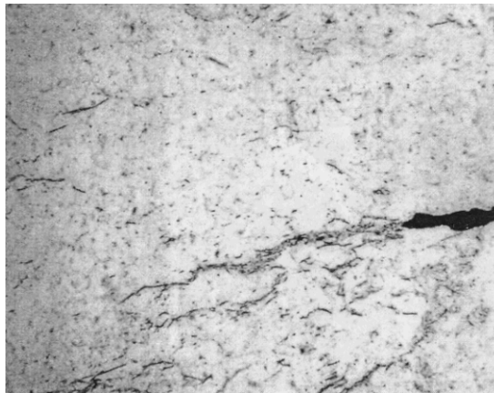
Figure A9.1 Orientation of Hydrides & Formation of The Hydride Cluster Near Crack
