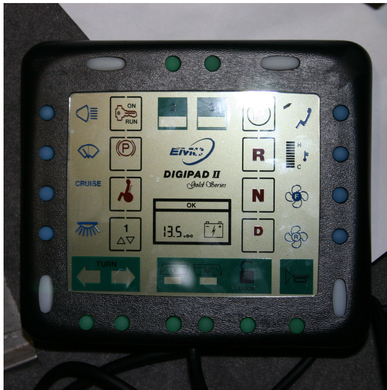
Figure 9: EMC control panel for secondary functions
