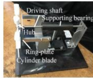
(b) Structure of rotation mechanism at un-loaded condition for d=20\text{mm} , l=60\text{mm} and N=8
