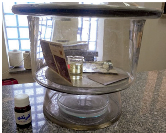
Figure 3. Exposure of the samples to the essential oil vapors using a desiccator.
