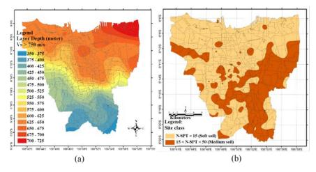
**Figure 1** Contour map of Jakarta: (a) depth of bedrock based on microtremor array measurement conducted by Ridwan *et al.* [4], (b) site classification based on SNI-1726-2012 by Irsyam *et al.* [3].
