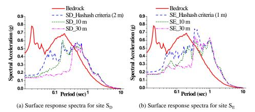
**Figure 8** Surface response spectra due to the effect of layer thickness for a megathrust earthquake with a return period of 2500 years scaled at a spectral period of 0.0 s.
