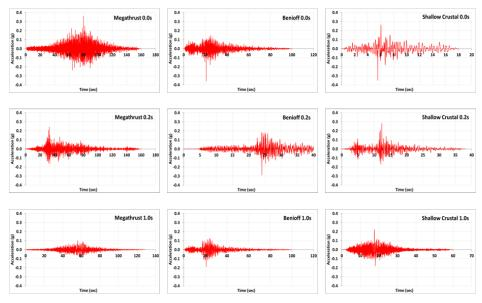
**Figure 4** Modified acceleration time histories on bedrock for Jakarta from megathrust, benioff, and shallow crustal earthquake sources for a return period of 2500 years (modified from Delfebriadi, *et al.* [22]).
