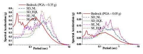
(a) Surface response spectra for PGA 0.35 g (b) Surface response spectra for PGA 0.05 g
