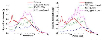
(a) Surface response spectra for site  $S_D$  (b) Surface response spectra for site  $S_E$
