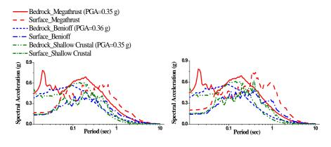
(a) Surface response spectra for site  $S_{\rm D}$  (b) Surface response spectra for site  $S_{\rm E}$
