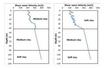
(a) Site  $S_D$  for depth up to 40 m (b) Site  $S_E$  for depth up to 40 m
