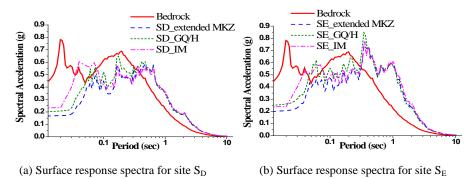
**Figure 6** Surface response spectra of the three soil models for a megathrust earthquake with a return period of 2500 years scaled at spectral a period of 0.0 s.
