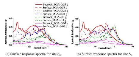
**Figure 14** The surface response spectra of several *PBAs* of input motion due to a megathrust earthquake with a return period of 2500 years.
