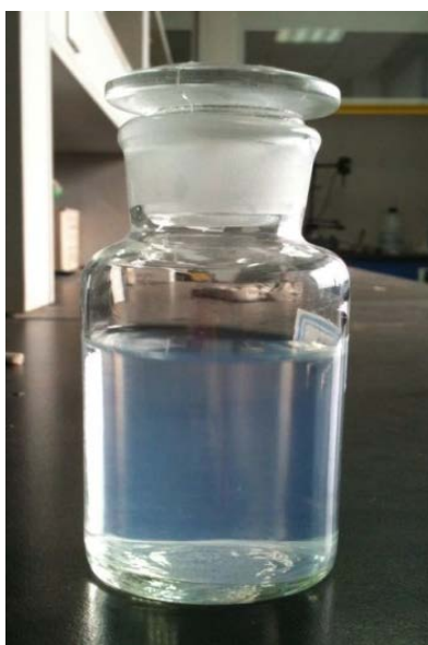
Figure 1 Silica sol prepared by Stöber method.
