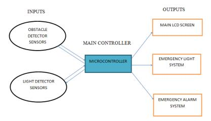
Figure 1 Block diagram of proposed system.
