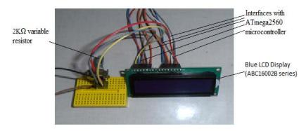
Figure 3 Blue LCD display set up.
