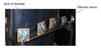
Figure 14 Installation of 5 ultrasonic sensors.
