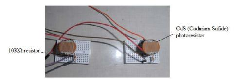
Figure 8 Light detection sensor.
