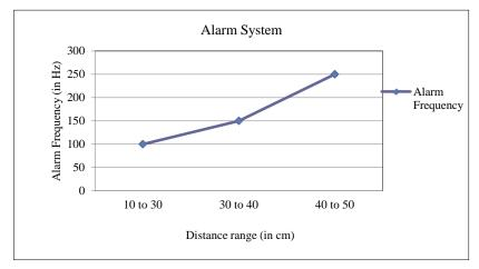
Figure 15 Distance vs alarm frequency.
