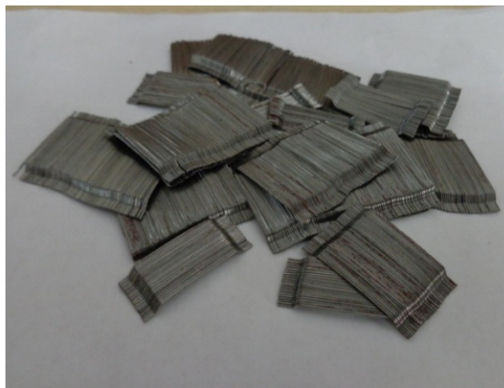
Figure 2 Snapshot of glued steel fibers.
