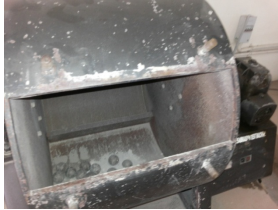
Figure 1 Mechanical grinding of fly ash.
