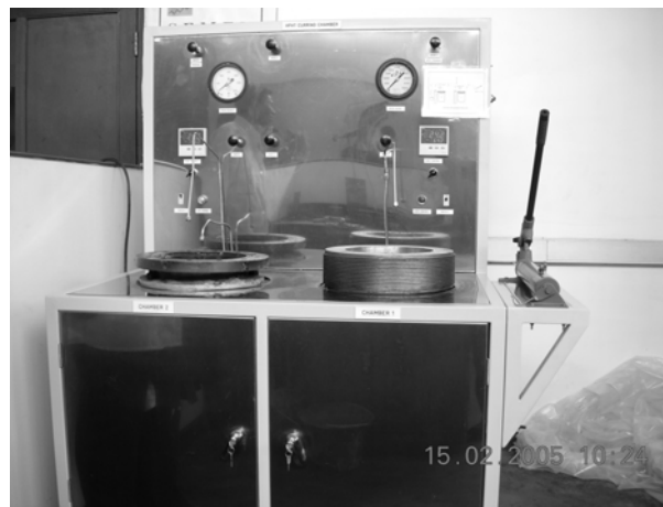
Figure 3.1 Modified HPHT Curing Chamber.
