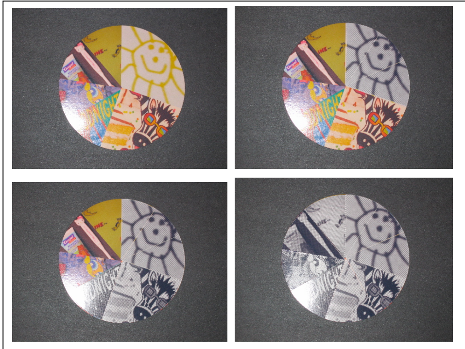
Figure 4. Prototype lightweight display of to-do list on pie chart. Four chapters from top left: start of timer shows full image of entire “pie”; after 15 min., 1/3rd of image turns black and white; after 30 min., only 1/3 of original color image remains on display; final image is all black and white... bedtime!
