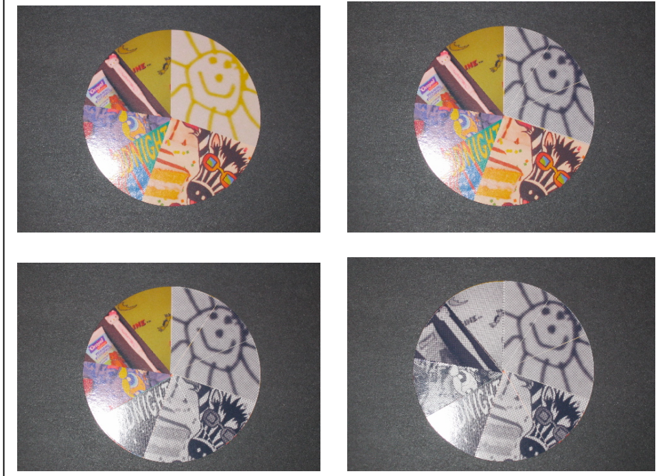
Figure 2. Table 1, Prototype lightweight display (a): to-do list on pie chart. Task images on pie slices in order of bedtime routine; overlay different pie slice on top of image every 5 min. (15 min. in this illustration) to show the time slice is up.
