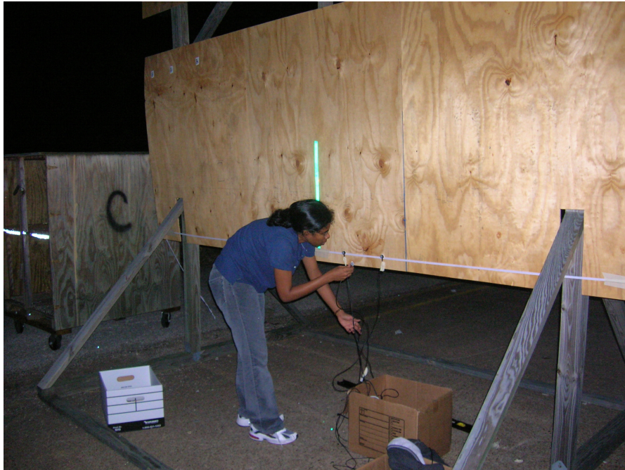
FIGURE IV.4 Placement of Illuminance Meter Sensors on Measuring Screen
