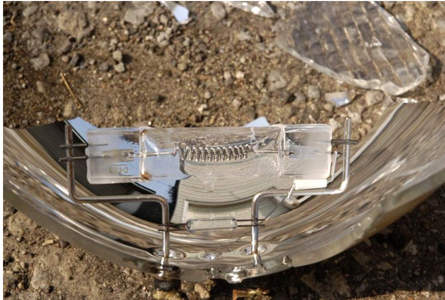
FIGURE II.5 Filament in a Sealed Beam Headlamp (22)
