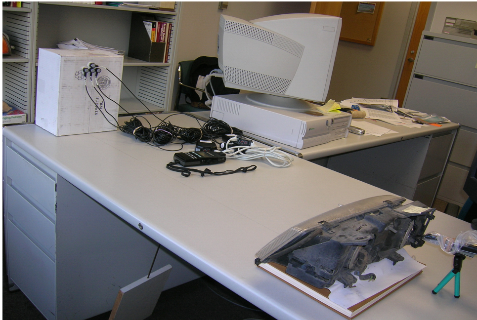
FIGURE V.1 Test Setup for Headlamp Degradation Test
