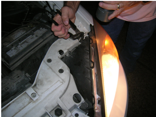
(a) Adjustment of the Vertical Aiming Screw
