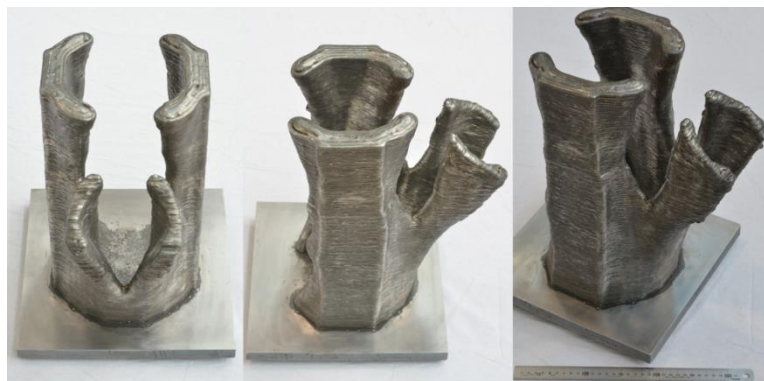
Figure 8. Additively manufactured, topology-optimized 30° oblique joint.
