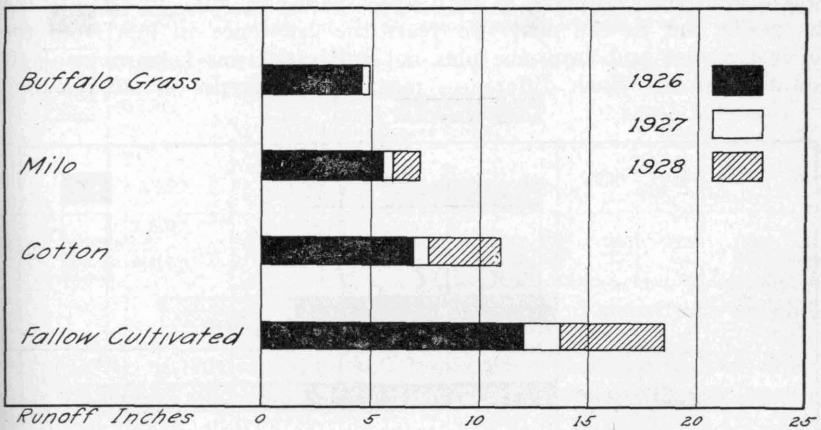
Fig. 19. Influence of crop on runoff from land with a 2 per cent grade.
