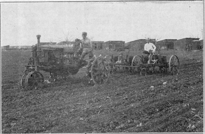
Figure 4.—Four-row outfit which plants from 35 to 40 acres per day.
