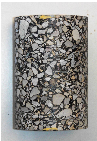
Figure 3.3: Example of Trimmed Specimen for Flow Number Test (Glacial Gravel).
