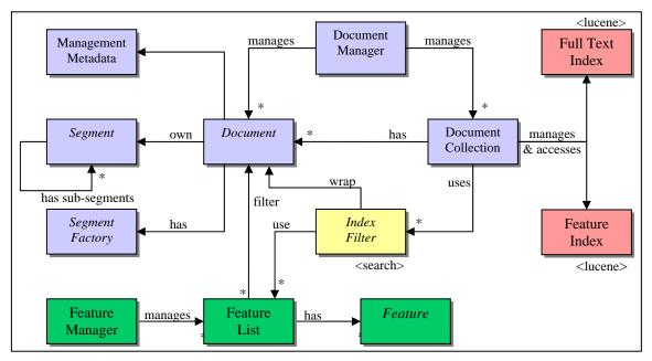
Figure 2: Structural components of the feature identification framework
