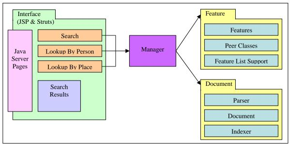
Figure 14: The architecture of the Sliwa application
