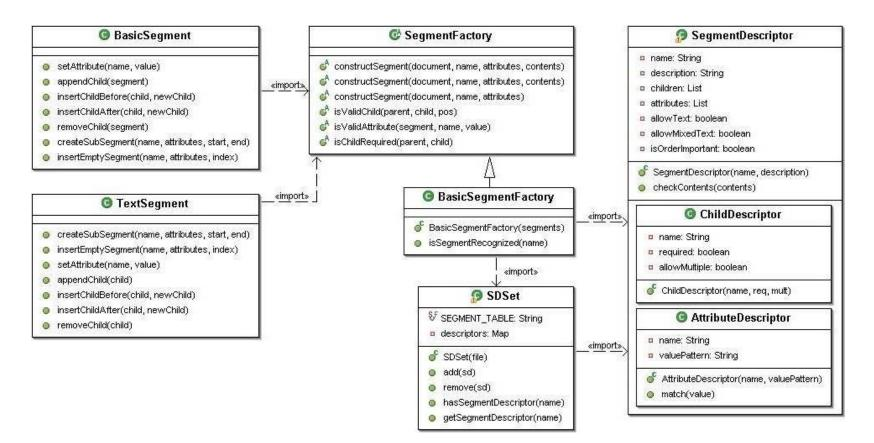
Figure 6: Class diagram of the default segment factory implementation
