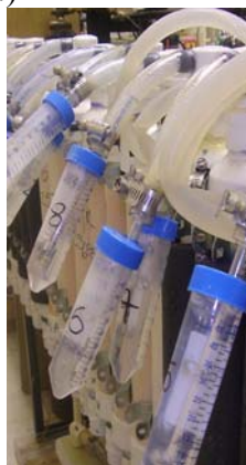
Fig. 7. Reactor system. a) Complete system. b) Reactors at 55 and 65°C were coated with insulating material. c) Temperature controller. d) Flow rate of gasses measured as bubbles per second. e) Bottle with lime slurry to scrub CO 2 in the air.
