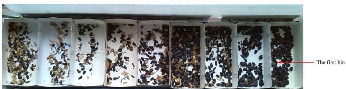
Figure 2 The sample of seed sunflower separation in the best treatment combination 60 rpm, 6cm and 20 kV
