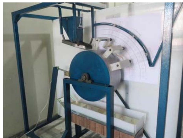
Figure 1 A laboratory roll-type corona separator
