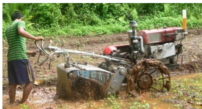
Figure 2 Power tiller fitted with cage wheel having newly developed lugs
