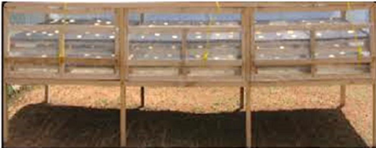
Figure 3 NRI Kawanda cabinet solar dryer ( Wakjira et al., 2011)
