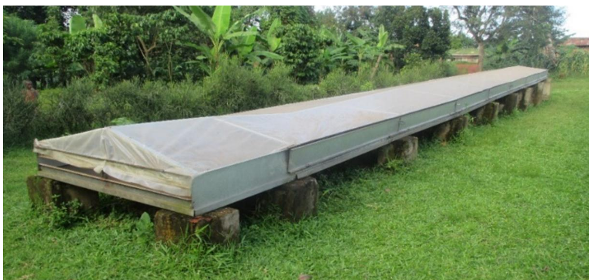
Figure 2 PPI tunnel solar dryer model (Credits Galyaki, C)
