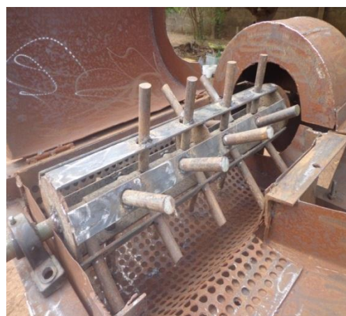
Figure 2 Threshing chamber of soybean threshing machine consisting of spike tooth beaters, screen, disc bar, flat bar, shaft and bearings
