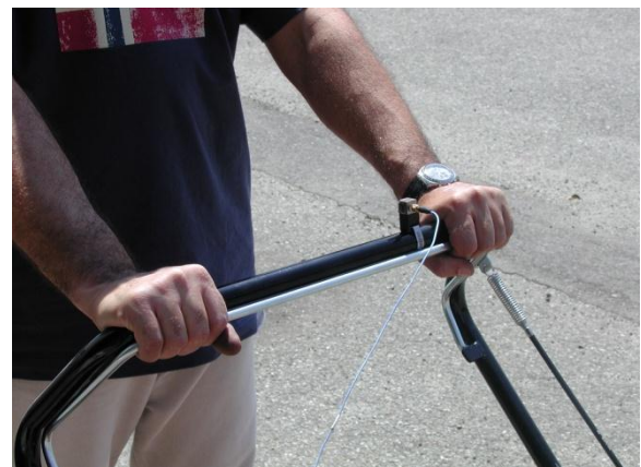
Figure 2 Accelerometers fastened to the handlebar of the mower for vibration data acquisition
