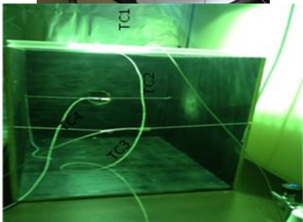
Figure 1 Testing setup showing the black box, full spectrum light and the positions of the used thermocouples
