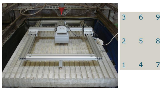
Figure 3 Schematic representation (right) of the nine locations at the floor element (left)
