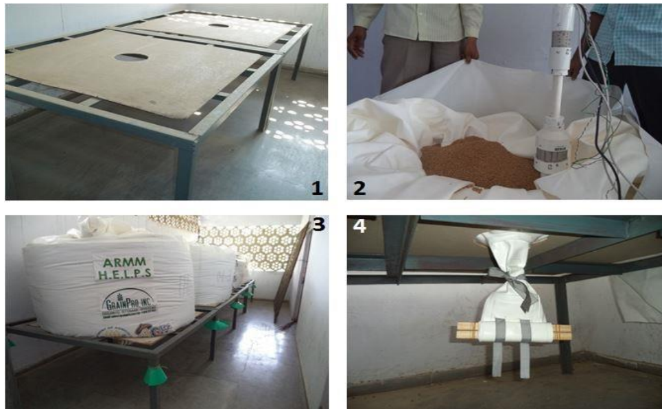
Figure 1 A view of table shaped metallic frame (1), sensor rod installation (2), final experiment setup with rat cone (3) and drain tube (4) of the hermetic bags.
