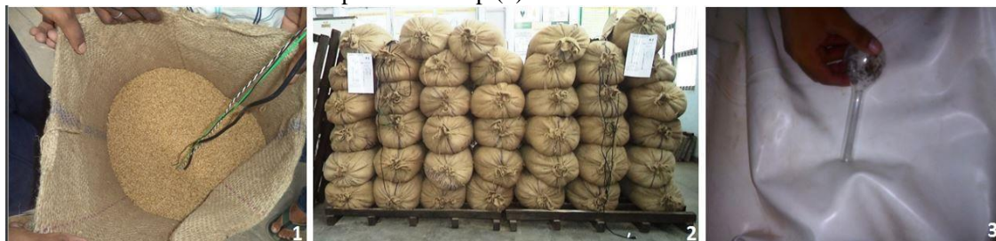
Figure 3 A view of sensor rod installation in gunny bag (1), Gunny bags piles on wooden crates (2) and manual insect infestation (3) of the hermetic bag.
