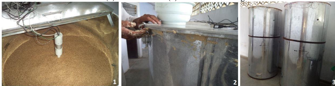
Figure 2 A view of sensor rod installation (1), sealing of infiltration with wheat flour paste (2) and final experiment setup (3) of the steel bins.
