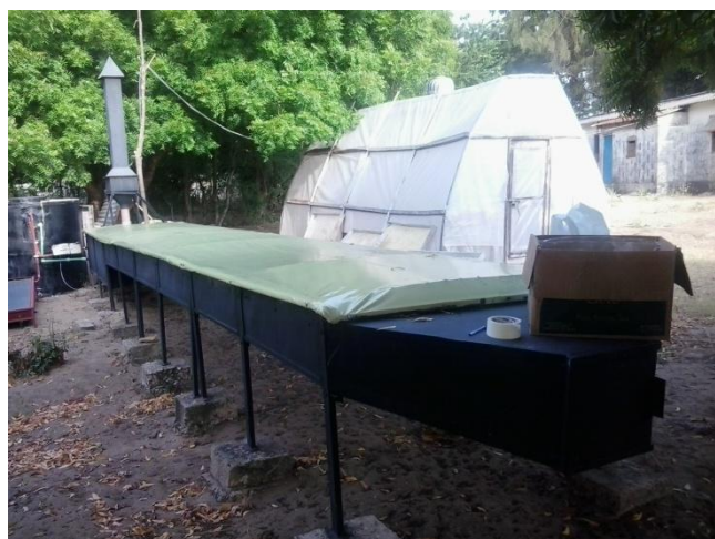
Figure 1 The hybrid solar-windmill solar tunnel dryer
