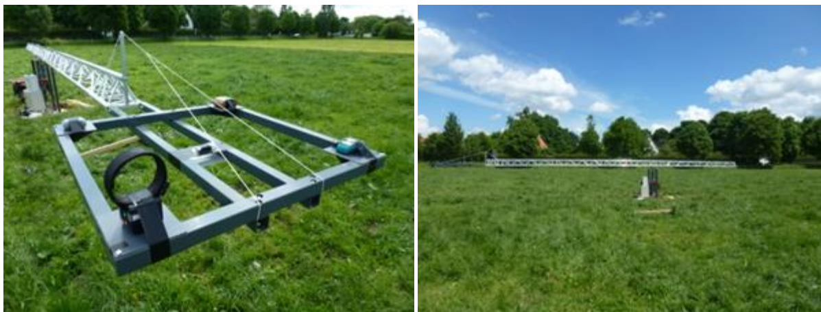
Figure 2 Rotating dynamic test apparatus for testing the dynamic accuracy of GNSS receivers and a data logger
