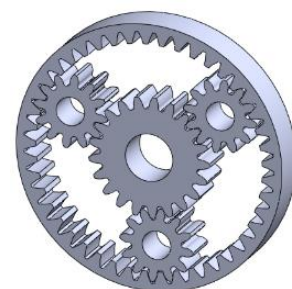
Figure 5 Isometric view of final drive
