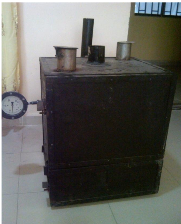
Figure 1 Front view of the charcoal fuelled cabinet dryer
