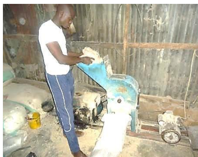
Figure 3 Grinding operation using a hammer mill
