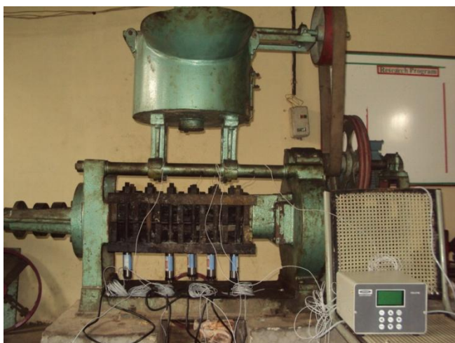
Figure 4 The experimental set: Oil expeller fitted with temperature and pressure transducer
