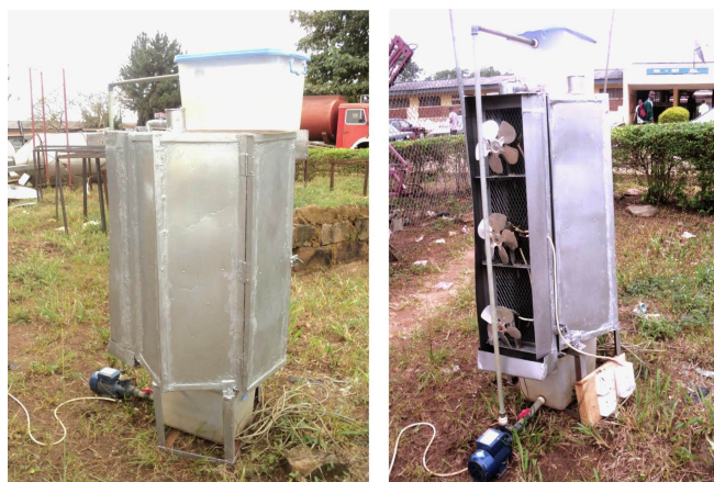
Figure 1 Prototype developed active evaporative cooler
