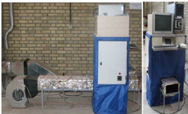
Figure 2 Photographic view of the experimental dryer
