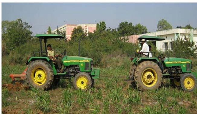
Figure 3 Measurement of draft of the implement during the field experiments
