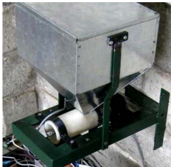
Figure 1 Fertilizer hopper and metering screw assembly used for laboratory and field tests
