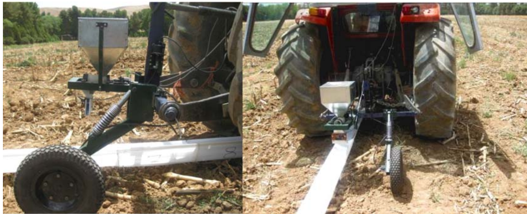
Figure 2 Two views showing the components of ground-driven wheel used for measurement of tractor travel speed and displacement.
