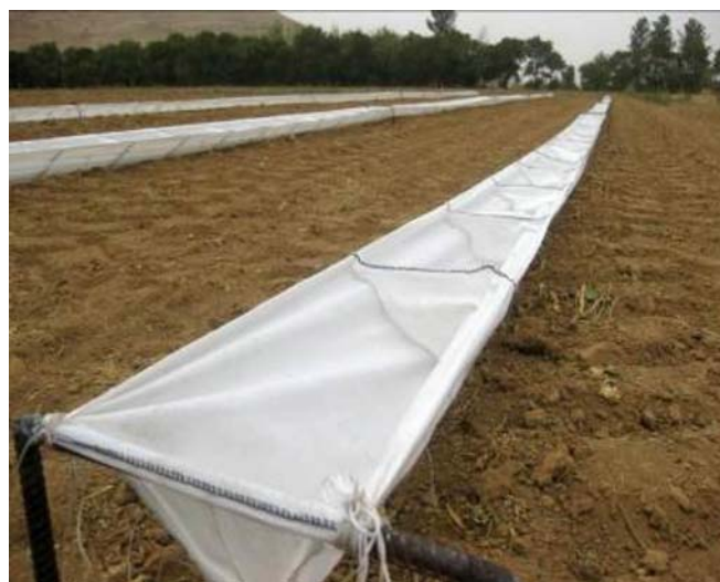
Figure 5 Arrays of patternators made of canvas for measuring the discharge rate of fertilizer along each planting row. Each array was made up of thirty 50 cm long, 25 cm wide buckets
