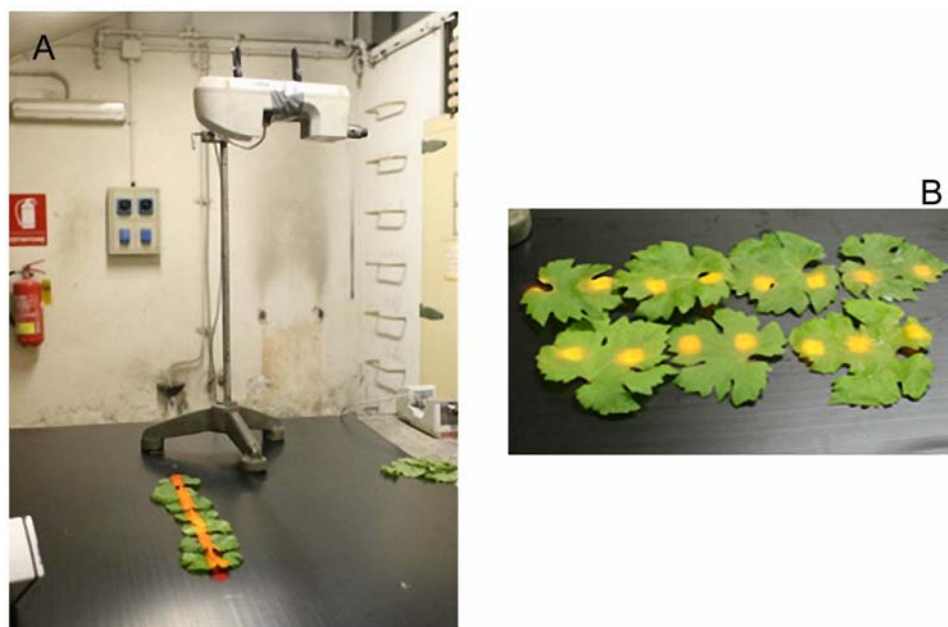
Figure 2. A) The metallic bar used as support for GreenSeeker and Crop Circle during the measurements. The red line represents the light emitted by GreenSeeker. B) The field of view of Crop Circle consists of 15 spotlights.
