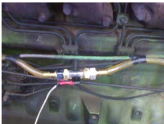
Figure 5. A view of a flow meter in contact with the engine to study the effects of vibration.
