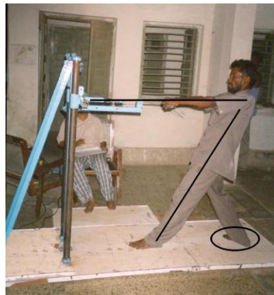
Fig. 2 Measurement of pull force with both hands in standing posture in horizontal plane
