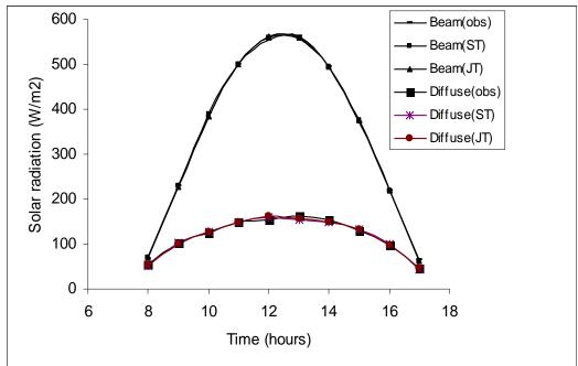
Fig 3(a) Hourly variation in beam and diffuse radiation with time for the month of January (weather type 'b') using cloudiness/haziness factor and atmospheric transmittances
