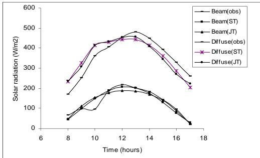
Fig 5(b) Hourly variation in beam and diffuse radiation with time for the month of June (weather type 'd') using cloudiness/haziness factor and atmospheric transmittances
