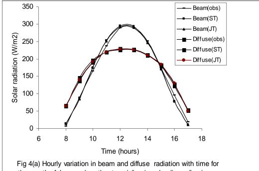
Fig 4(a) Hourly variation in beam and diffuse radiation with time for the month of January (weather type 'c') using cloudiness/haziness factor and atmospheric transmittances
