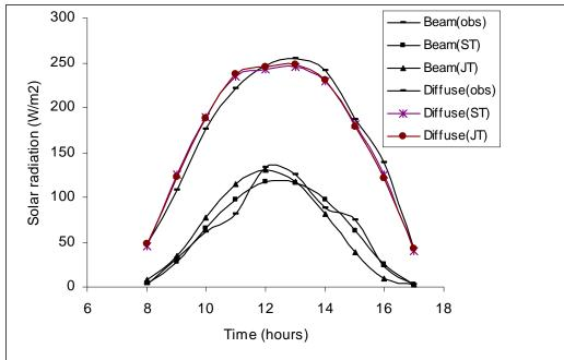
Fig 5(a) Hourly variation in beam and diffuse radiation with time for the month of January (weather type 'd') using cloudiness/haziness factor and atmospheric transmittances
