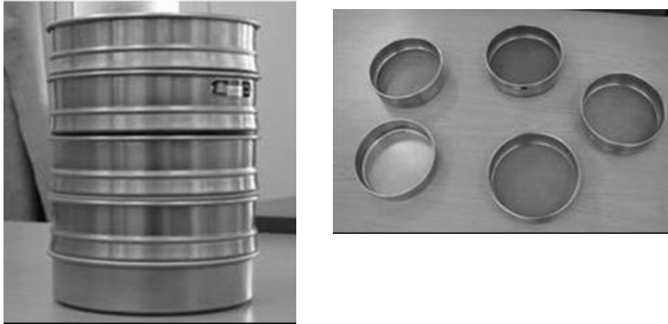
Figure 2. Sieve box and sieves used in the experiments
