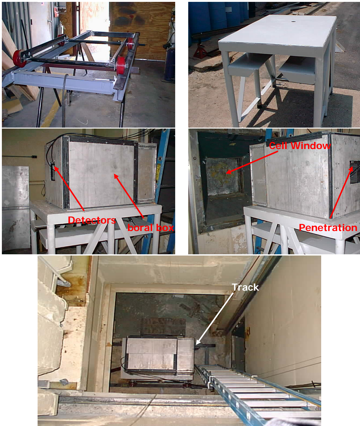
Fig. 2.10. Components used to set up the exposure cave inside the irradiation cell, and final setup of the FNIS including the exposure cave, movable working table, track, and detectors installed inside the irradiation cell.
