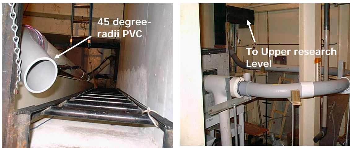
Fig. 2.13. Sample transfer system installed in the upper research level and in the irradiation cell for sample loading/unloading and exposure control.
