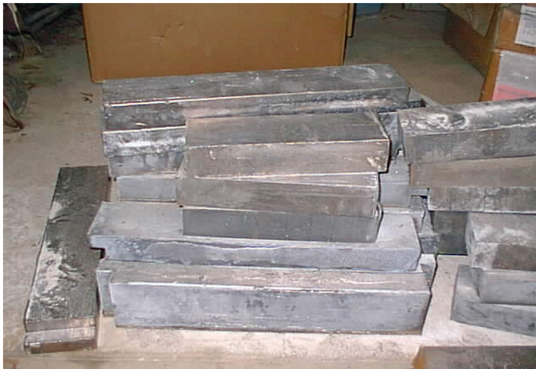
Fig. 2.5. Lead-bismuth ingots, which contains 44.5 w % lead (Pb) and 54.9 w % bismuth (Bi), and lead-bismuth bricks for the FNIS setup, which have the size of 10.16 cm × 48.26 cm × 5.08 cm.
