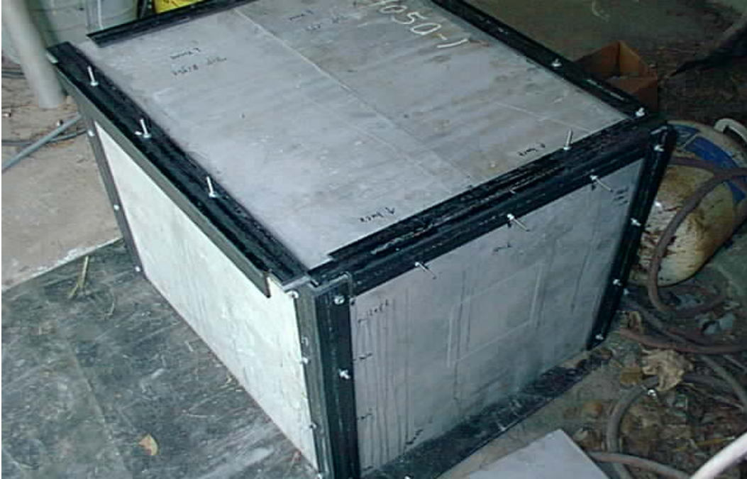
Fig. 2.8. Boral box constructed for shielding against thermal neutrons.
