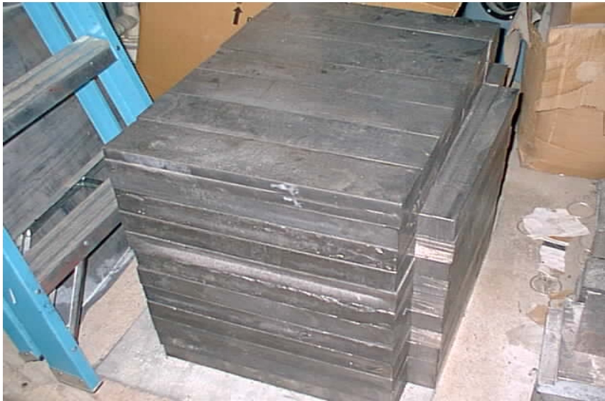
Fig. 2.9. Exposure cave for sample irradiation, which was constructed with the lead-bismuth bricks.
