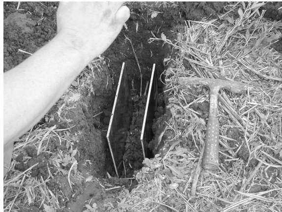
Fig. 7.11. Two aluminum plates buried in the VVP configuration in Brazos County, Texas.
