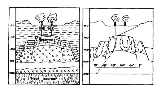
Fig. 1. Scheme of an ideal geothermal field according to Tonani et al., 1964.
