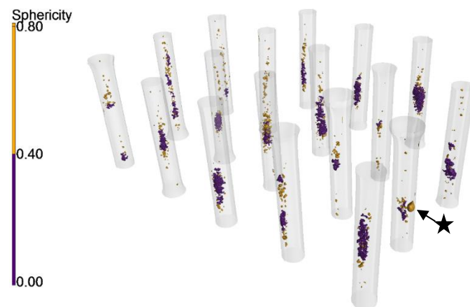
Fig. 8.4 3D visualisation of porosity within the gauge length of tensile specimens obtained via X-ray tomography. Each connected pore is designated a colour based on its sphericity. Pores of sphericity greater than 0.4 were believed to originate from gaseous sources, whilst those of sphericity below 0.4 were attributed to solidification shrinkage or oxide films.
