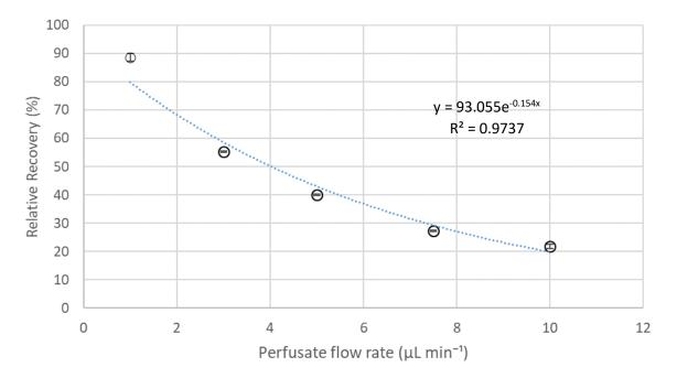
**Figure 1.** The effect of perfusate flow rate ( $\mu$ L min<sup>-1</sup>) on relative recovery (%) of Cr<sup>VI</sup> (100  $\mu$ g L<sup>-1</sup>) in stirred solutions (n = 5 for each flow rate). Exponential trendline and correlation coefficient (R<sup>2</sup> = 0.9737) are displayed within the chart. Error bars indicate  $\pm$  standard error from 5 replicates.
