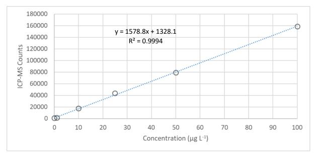
**Figure 2.** Calibration curve ( $R^2 = 0.9994$ ) for online MD-HPLC-ICP-MS system at nominal concentrations of 1, 10, 25, 50 and 100  $\mu$ g L<sup>-1</sup>. MD probes were immersed in 50 mL plastic beakers containing  $Cr^{VI}$  solution, stirred and perfused at 3  $\mu$ L min<sup>-1</sup>.
