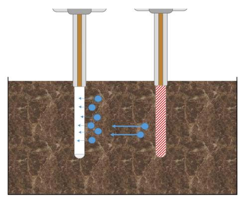
Figure 4. Diffusion of solutes (blue circles) towards probes implanted in soil matrix. Reduced permeability (represented by diagonal fill) in right MD probe shifts the diffusion gradient towards the left MD probe, therefore the right MD probe will sample lower concentrations of solute.
