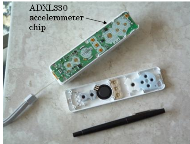
Figure 1. The Wii controller, inside-out. (Top) Broken open we see a (4-layer) circuit board and some standard switches. (Below) The famous accelerometer does not occupy a central location in the controller.
