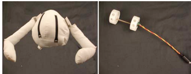
Fig 3: TUI3D: Uniball interface (left); various limbs with own sensors (see right) can be plugged into a central interface controls the virtual character in the Unreal engine (right)
