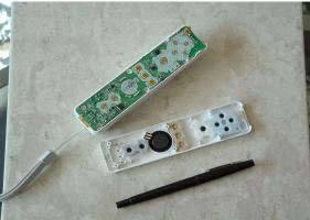
*Figure 3*: The *Wii* controller, inside-out. Left: The famous accelerometer does not occupy a central location in the controller. Right: broken open we see a (4-layer) circuit board and some standard switches (buttons!).
