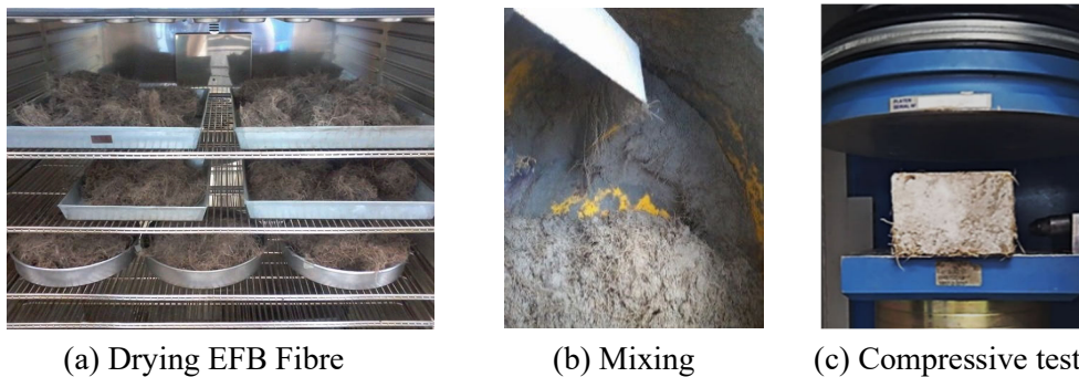
Fig. 1. Preparation and testing of the specimens
